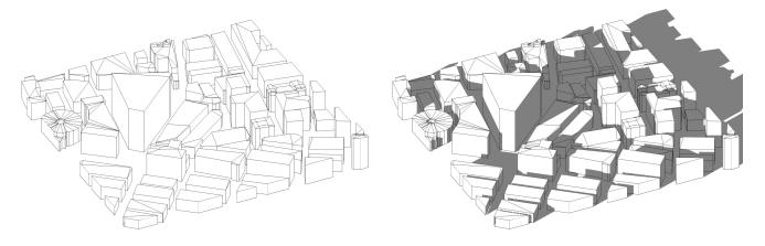
**Figure 4:** A section of the three-dimensional model (left) with sample image of shadow information (right)
