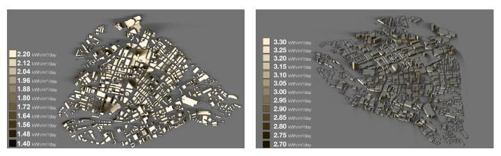
Figure 6: Completed roof top shadow map for March (left ) and completed south-east facade map for June (right)
